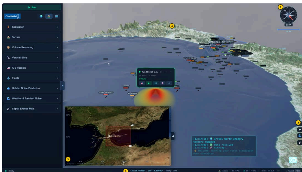
Figure 9.1 Terrain mode after the guest demo run. (1) Compass and scale bar. (2) Weather and signal-excess toggles. (3) Navigation minimap. (4) Amber depth-axis handle. (5) Scene centre and water depth in the status bar.
